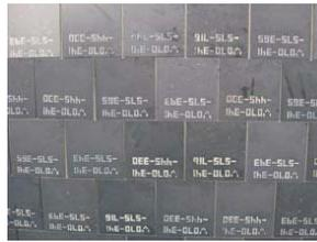
**Fig.2** Insulation tiles on the lower side of the wings of Shuttle model *Explorer*
